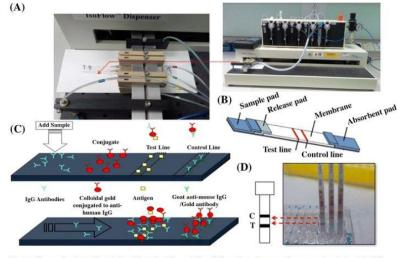
Preparation and schematic of lateral flow dipstick. a Jetting it linearly onto a membrane card using IsoFlow<sup>™</sup> Dispenser, b a lateral flow device in the dipstick format, c operation principle of a lateral flow dipstick, and d expected results of a lateral flow dipstick
